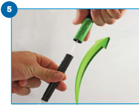
5 Withdraw the swab by gently pulling and twisting the swab handle.
