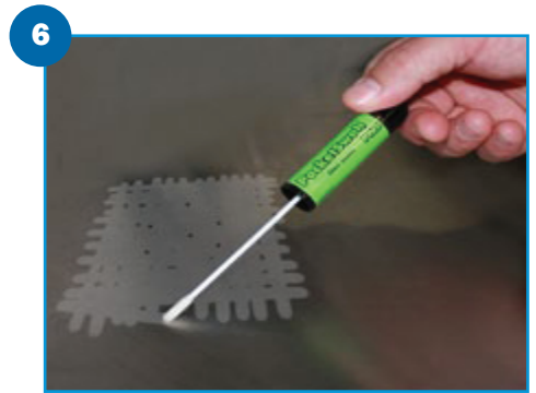
6 Swab an area 100 cm 2 (16 in 2 ). Rotate the handle to achieve full swab contact with surface.
