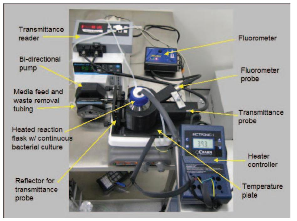
Figure 1 Legend: 60 - 150 ml bacterial culture in a disposable flask in probe holder on a heated base plate at 38°C. Media/water-sample mix is fed in and culture removed at the same rate using disposable tubing and external transmittance probe-reflector with computer software (not shown). External fluorometer probe detects coliphage infection of culture.
