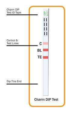
Charm<sup>®</sup> technology is trusted by the dairy industry worldwide for fast and accurate milk residue screening. The **Charm MRL Beta-lactam and Tetracycline DIP Test** detects Beta-lactam and Tetracycline drugs in raw commingled milk. The test follows a one-step procedure. Simply dip the strip into the sample and visually interpret within minutes.
